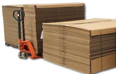
**Corrugated fanfold bales stack and store easily. The bales feed into a BOD® machine to produce right-sized boxes on demand.**
