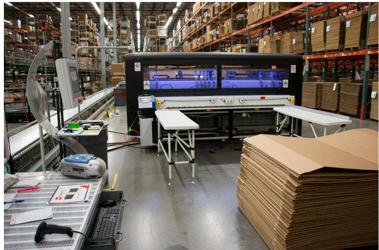
**Box On Demand® box making machine Compact 3.0 with integral ILG5 Gluer and Matrix™ Dimensioning Scan Table.**
