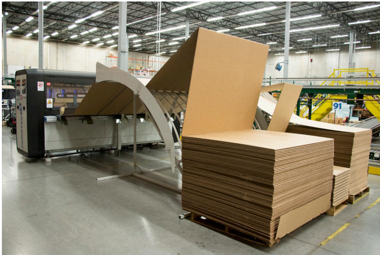
Corrugated Fanfold provided for a Box On Demand<sup>®</sup> machine in widths designed to optimize box size and type
